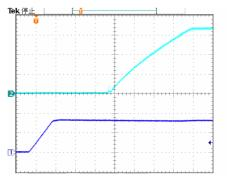
Figure 7: Turn-on transient at zero load current (4 ms/div). Vin=48V. Top Trace: Vout, 1.0V/div; Bottom Trace: Vin. 30V/div
