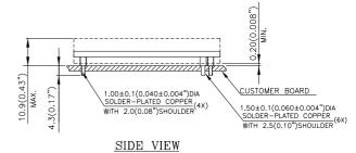
\*PIN1,3,4,5,9,10 ARE 1.50(0.060") DIA \*PIN2,6,7,8 ARE 1.00(0.040") DIA
