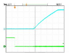
Figure 5: Turn-on transient at zero load current (4 ms/div). Vin=48V. Top Trace: Vout: 1.0V/div, Bottom Trace: ON/OFF input, 2V/div
