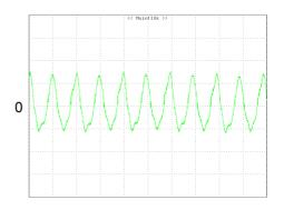
**Figure 11:** Input Terminal Ripple Current, i<sub>c</sub>, at full rated output current and nominal input voltage with 12μH source impedance and 100μF electrolytic capacitor (200 mA/div, 2us/div)
