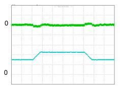
Figure 8: Output voltage response to step-change in load current (75%-50%-75% of lo, max; di/dt = 0.1A/µs). Load cap: 10µF tantalum capacitor and 1µF ceramic capacitor. Top Trace: Vout (100mV/div, 200us/div), Bottom Trace: lout (20A/div). Scope measurement should be made using a BNC cable (length shorter than 20 inches). Position the load between 51 mm to 76 mm (2 inches to 3 inches) from the module
