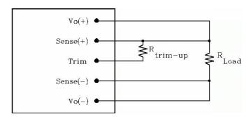
Figure 18: Circuit configuration for trim-up (increase output voltage)
