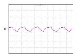
Figure 14: Output voltage ripple at nominal input voltage and rated full load current (100 mV/div, 1us/div)
