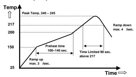
Note: The temperature refers to the pin of E48SP, measured on the pin +Vout joint.
