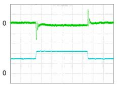
**Figure 9:** Output voltage response to step-change in load current (75%-50%-75% of lo, max; di/dt =  $1.0A/\mu s$ ). Load cap:  $10\mu F$  tantalum capacitor and  $1\mu F$  ceramic capacitor. Top Trace: Vout (100mV/div, 200us/div), Bottom Trace: lout (20A/div). Scope measurement should be made using a BNC cable (length shorter than 20 inches). Position the load between 51 mm to 76 mm (2 inches to 3 inches) from the module
