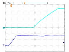
Figure 6: Turn-on transient at full rated load current (4 ms/div). Vin=48V. Top Trace: Vout, 1.0V/div; Bottom Trace: Vin . 30V/div
