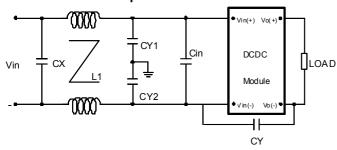
Cin is 100uF\*2 low ESR Aluminum cap; CX is 2.2uF ceramic cap; CY1 are 10nF ceramic caps; CY2 are 10nF ceramic caps;
